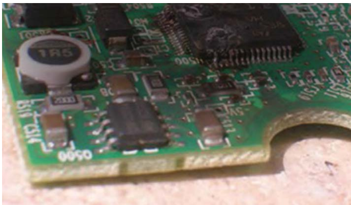
Transient overvoltage effect
